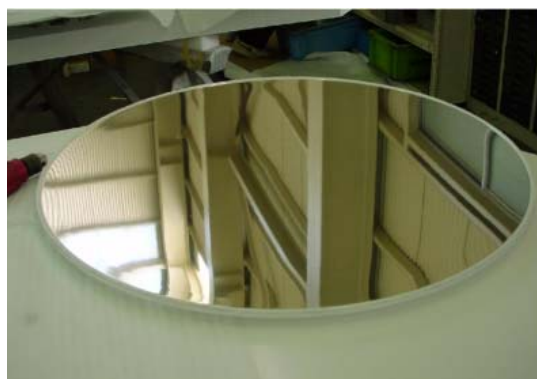
Figure 4.5 GFRP mirror segment with 80 cm diameter and 5 kg weight.
