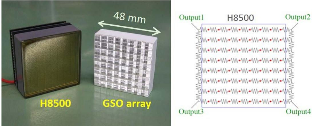
Figure 5.14: (Left) Multi-anode photomultiplier Hamamatsu H8500 and pixel scintillation array of GSO crystal ( $8 \times 8$  pixels). (Right) Schematic view of the resistor matrix attached to a PSA, which has 64 inputs from a PSA (red circle) and 4 outputs of divided charge at the corner (Mizumoto et al., 2015).
