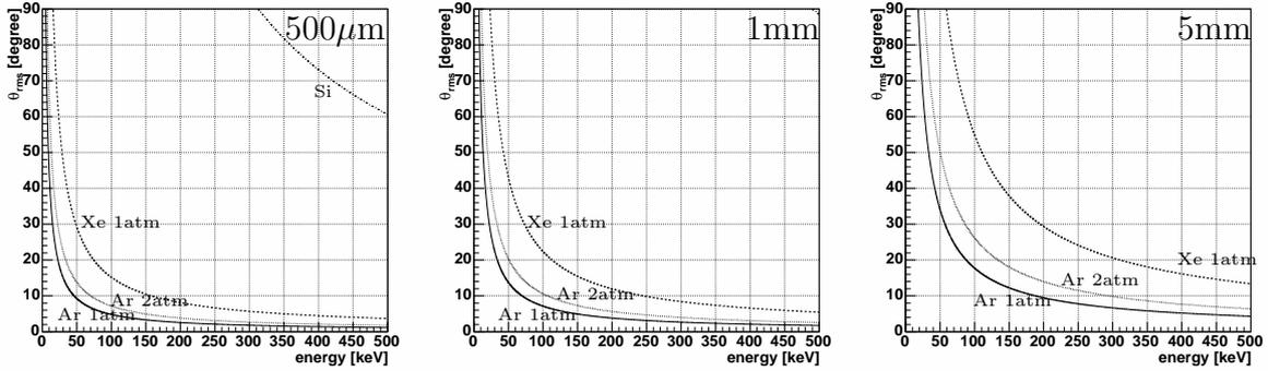
Figure 5.3: Scatter angle deviation with different ranges of the electron (left:  $500\mu\text{m}$ , middle:  $1\text{mm}$ , right:  $5\text{mm}$ ; temperature:  $20^\circ\text{C}$ ; [Takada 2007](#)).
