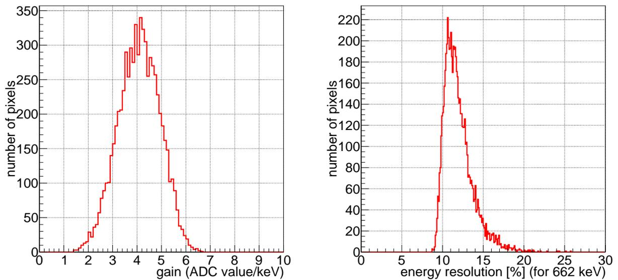
Figure 5.16: (Left) Gain distribution of the whole channels of the scintillation camera. The unit of the gain is ADU/keV and divided by the average. (Right) the same but for the energy resolution at FWHM for 662 keV (Mizumoto et al., 2015).
