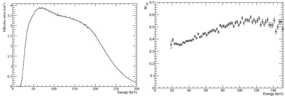
Figure 4.12: (Left) Effective area of PoGO+. (Right) Simulated modulation factor as a function of energy. Figures from [Chauvin et al. \(2017\)](#).
