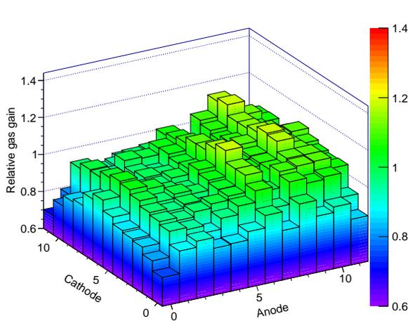
Figure 5.11: Gas gain map of the TPC. Color maps represent the relative gas gain with respect to the mean gas gain of the whole region (Sawano, 2017).
