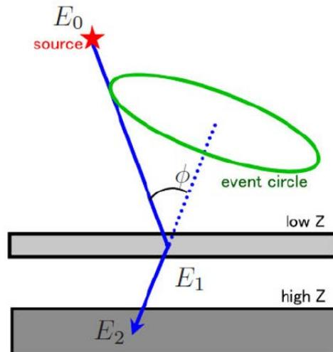
Figure 4.17: Schematic view of Compton cameras (Takada, 2007).
