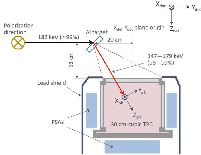
Figure 7.10: A side view in the  $Y_{det}-Z_{det}$  plane of the ETCC setup for the second experiment on BL08W at SPring-8. The Al target was shifted 20 cm into the upper stream of the beamline than in the previous experiment. The photon coordinate system  $X_{ph}Y_{ph}Z_{ph}$  has the  $Z_{ph}$ -axis along the average direction of the incident photons, and the  $X_{ph}$ -axis coincides with the  $X_{det}-Y_{det}$  plane. Figure adapted from [Komura et al. \(2017\)](#).
