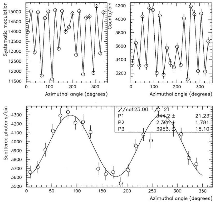
Figure 3.5: Azimuthal angle distributions of scattered photons calculated by the Monte Carlo simulation of COMPTEL; top left) unpolarized incident photons,  $\mathcal{N}_{\Pi=0}(\phi_{det})$ ; top right) completely polarized photons,  $\mathcal{N}(\phi_{det})$ ; bottom) corrected distribution,  $\mathcal{N}_{cor}(\phi_{det})$  and its best fit with  $\cos(2\phi_{det})$  function. The incident photons are on-axis with energy of 1 MeV (Lei et al., 1997).
