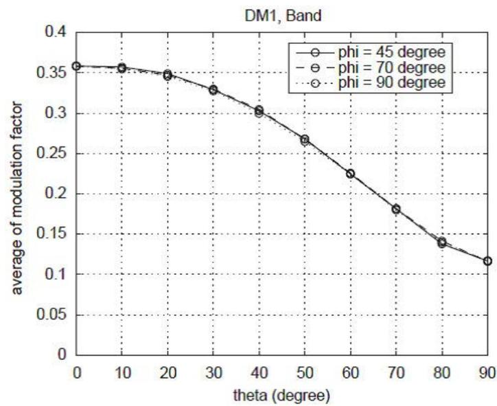
Figure 3.8: The simulated modulation factors of a certain model of POLAR detector. They varies with incident angle  $\theta$  but remains almost constant with polarization angle  $\phi$  (Xiong et al., 2009).
