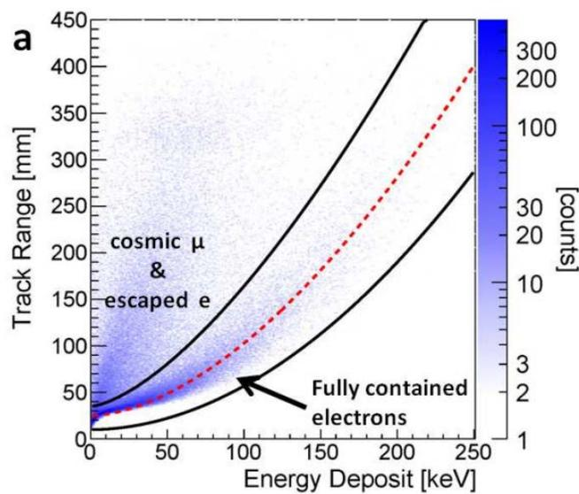
Figure 5.13: Track range vs the energy loss in the TPC under the condition of gamma-ray irradiation from  $^{137}\text{Cs}$  (3 MBq) at a distance of 1 m in the laboratory (Tanimori et al., 2015). The broken solid line represents the numerical calculation curves of the energy loss for fully-contained electrons.
