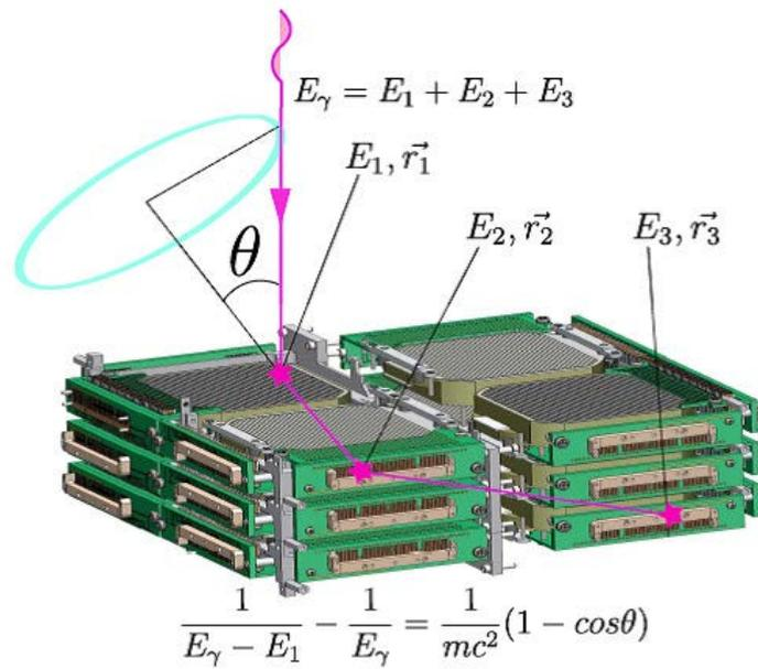
Figure 4.18: Schematic view of COSI detector (Chiu et al., 2015).
