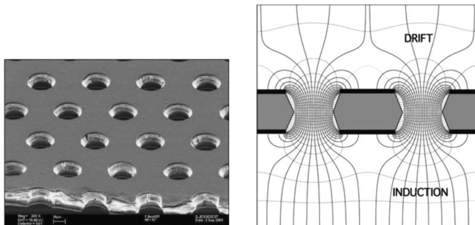
Figure 5.7: Gas Electron Multiplier electrode is a thin polymer foil, metal-coated on both sides and pierced with a high density of holes, typically  $50\text{--}100 \text{ mm}^{-2}$  (left panel). GEM electrode develops near the holes field lines and equipotential as shown in the right panel. The large difference of potential applied between the two sides of the foil provides the avalanche multiplication, and electrons are transferred into the lower section of the structure (Sauli, 2016).
