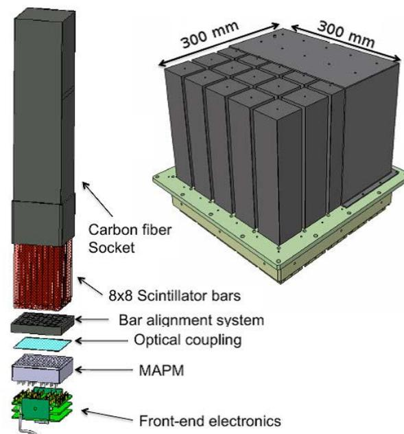
Figure 4.16: The schematic view of POLAR detector. Array of  $40 \times 40$  plastic scintillator bars (each  $5.8 \times 5.8 \times 172 \text{ mm}^3$ ), and bars grouped in 25 modules (Kole et al., 2016).
