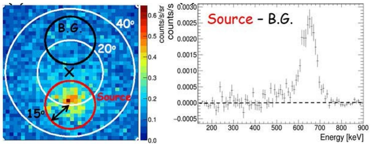
Figure 5.22: (Left) A image of  $^{137}\text{Cs}$  (2.9 MBq) source at the off-axis with a polar angle of  $20^\circ$ . Red and black circles, each of which is  $15^\circ$  in radius, indicate source and background regions, respectively. (Right) The spectrum after air-scattered gammas within the PSF ( $\sim 15^\circ$ ) are removed, using the region symmetrical about the centre of the FoV (black circle in left panel) as the background region (Tanimori et al., 2017).
