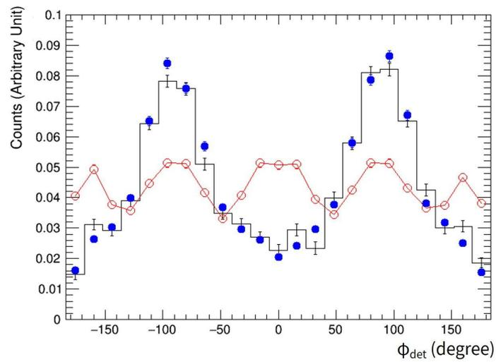
Figure 7.8: The solid line histogram represents the measured azimuthal angle distribution  $\mathcal{N}_{pol}^{mes}(\phi_{det})$ . The simulation results of the azimuthal angle distribution  $\mathcal{N}_{pol}^{sim}(\phi_{det})$  and  $\mathcal{N}_{unpol}^{sim}(\phi_{det})$  are plotted as filled circles and open circles, respectively. Figure adapted from Komura et al. (2017).
