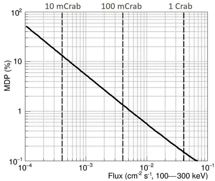
Figure 8.2: Solid line showing the calculated MDPs of the satellite-ETCC as a function of the source flux in the energy range of 100–300 keV for an observation time of  $10^7$  s. The dashed vertical lines represent source fluxes of 1, 1/10, and 1/100 the Crab nebula (Komura et al., 2017).
