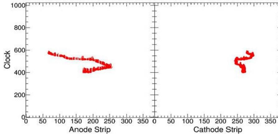
Figure 5.9: Typical examples of the projected track of a recoil electron, where both hit points are depicted. Since the drift velocity is  $8 \text{ cm}/\mu\text{sec}$ , 1 clock corresponds to  $0.8\text{mm}$ . In addition, the clock duration between rising and falling edges crossing the threshold is recorded as the time-over-threshold (TOT), which roughly corresponds to the deposited energy (Mizumoto et al., 2015).
