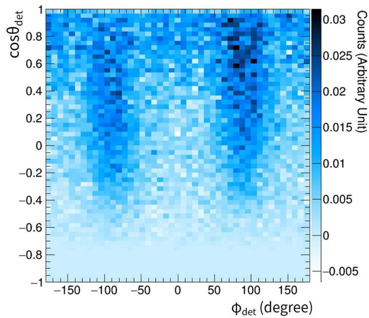
Figure 7.7: Two-dimensional scatter plot of the measured  $\mathcal{D}_{pol}^{mes}(\cos \theta_{det}, \phi_{det})$  when the polarization direction of the X-ray beam is  $0^\circ$ . Figure adapted from [Komura et al. \(2017\)](#).
