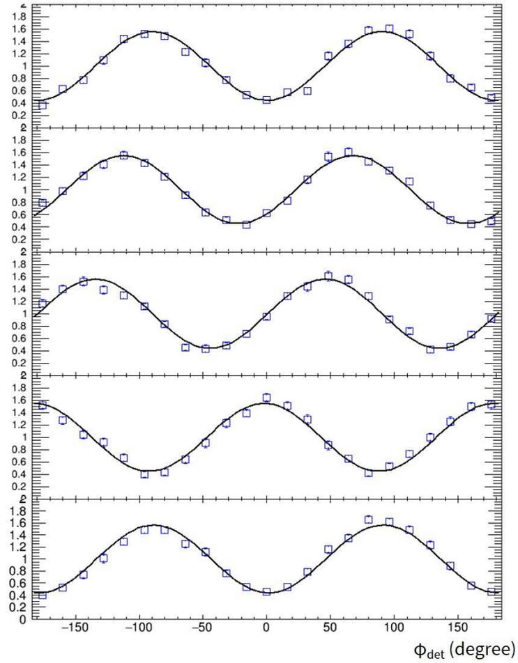
Figure 7.9: Corrected modulation curves (open squares) and the best fit curves (solid lines). The polarization direction of the X-ray beam is  $0^\circ$ ,  $-22.5^\circ$ ,  $-45^\circ$ ,  $-90^\circ$ , and  $-180^\circ$ , respectively, from top to bottom. Figure adapted from [Komura et al. \(2017\)](#).
