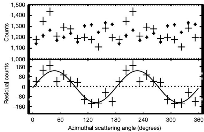
Figure 4.4: *RHESSI* observation of GRB 021206. The top panel shows both the measured scattered angle distribution (crosses) and the simulated scatter angle distribution (diamonds) for unpolarized radiation. The bottom panel shows the difference between the two distributions and the best-fit modulation curve, corresponding to a linear polarization of  $80 \pm 20\%$  (Coburn & Boggs, 2003).
