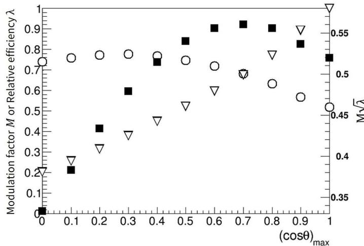
Figure 6.8: Dependences of the modulation factor  $M$  (open circles), the relative detection efficiency  $\lambda$  (open triangles), and the figure of merits  $M\sqrt{\lambda}$  (filled squares) on the integration region from 0 to  $\theta_{max}$ . Figure adapted from Komura et al. (2017).
