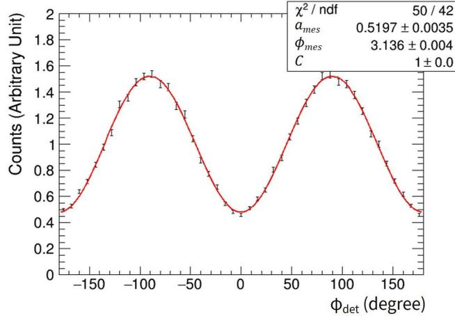
Figure 6.3: Corrected integrated azimuthal angle distribution of scattered photon  $\mathcal{N}_{cor}(\phi_{det})$  calculated from  $\mathcal{N}_{pol}(\phi_{det})/\mathcal{N}_{non}(\phi_{det})$ . Figure adapted from [Komura et al. \(2017\)](#).
