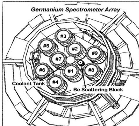
Figure 4.3: The *RHESSI* spectrometer array consists of nine Germanium detectors. Each Ge detector is 7.1 cm in diameter and 8.5 cm long (McConnell et al., 2004).
