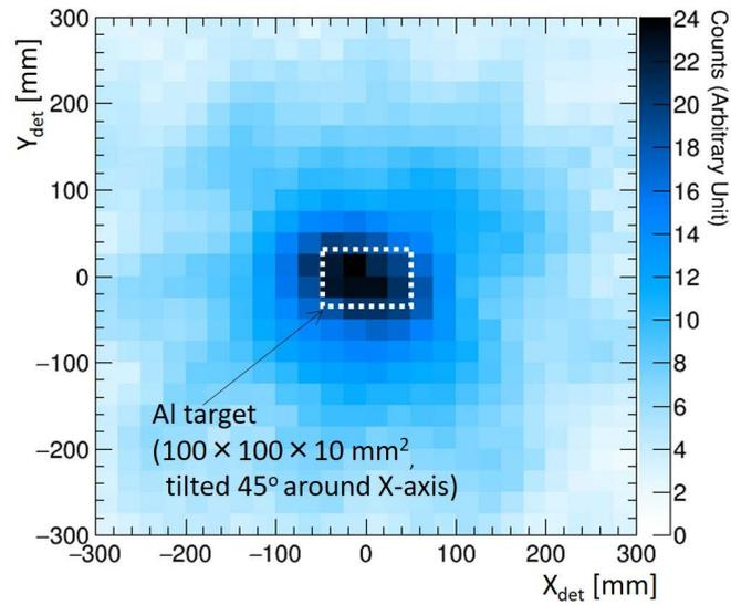
Figure 7.6: Reconstructed back-projection image of Al target.
