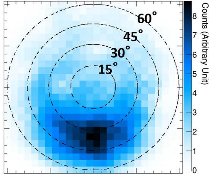
Figure 7.12: Reconstructed image showing the direction of an incident photon. The dotted concentric circles represent the incident angle ( $15^\circ$ ,  $30^\circ$ ,  $45^\circ$ , and  $60^\circ$ ) in the coordinate system of the ETCC. The spread in the image corresponds to the spread of the scattered beam. An enhancement is seen within the incident angles of  $20\text{--}40^\circ$ , and most events are concentrated near  $30^\circ$  (Komura et al., 2017).
