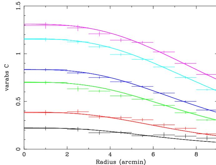
Figure 3: The time and positional dependence of contamination. Black, red, green, blue, light-blue, and magenta show the values of 2005/09 – 2006/02 in order. Solid lines mean results by applying the model shown as (3) to each month data.
