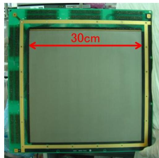
Figure 2. Picture of a large-sized  $\mu$ -PIC.
