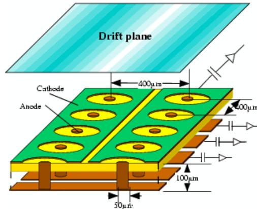
Figure 1. Structure of a  $\mu$ -PIC.
