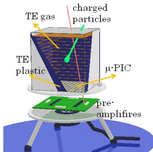
Figure 4. Design of the PS-TEPC.
