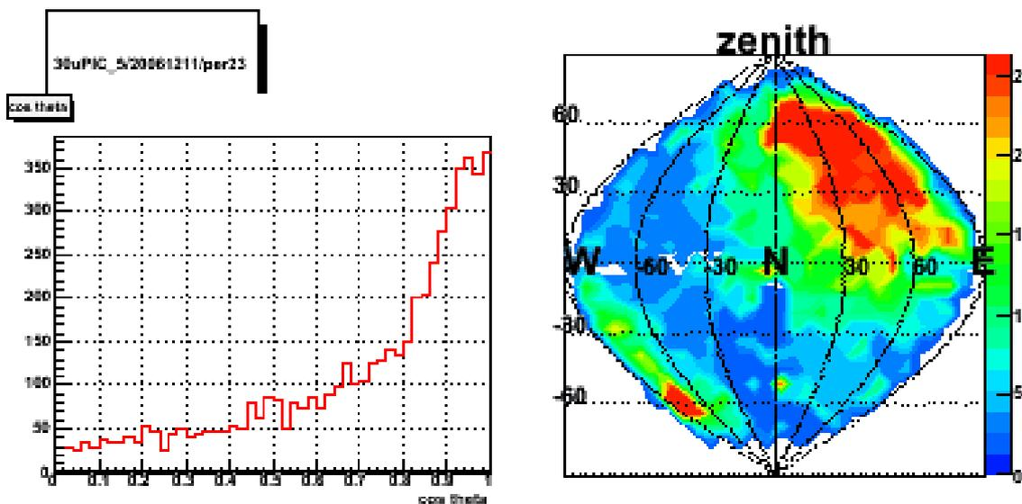
Figure 7. Measure  $\cos \theta$  distribution (left) and the neutron image drawn with the tracks of the recoil protons (right). Neutron source is set in the direction of 45 degrees from north to east and elevation of 35 degrees.
