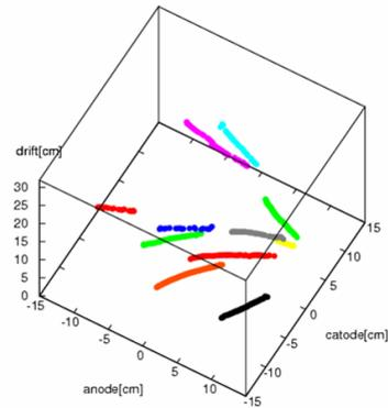
Figure 6. Proton tracks detected by a large-sized  $\mu$ -TPC.
