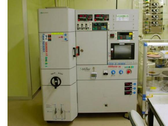
DC sputtering machine for Cu
