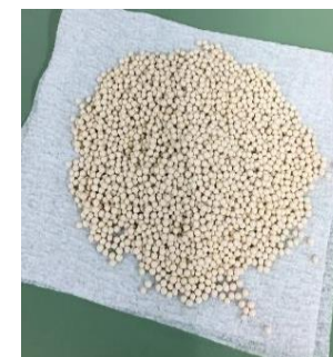
Zeolite: (\text{AlO}_2)_x \cdot (\text{SiO}_2)_y used as a molecular sieve
