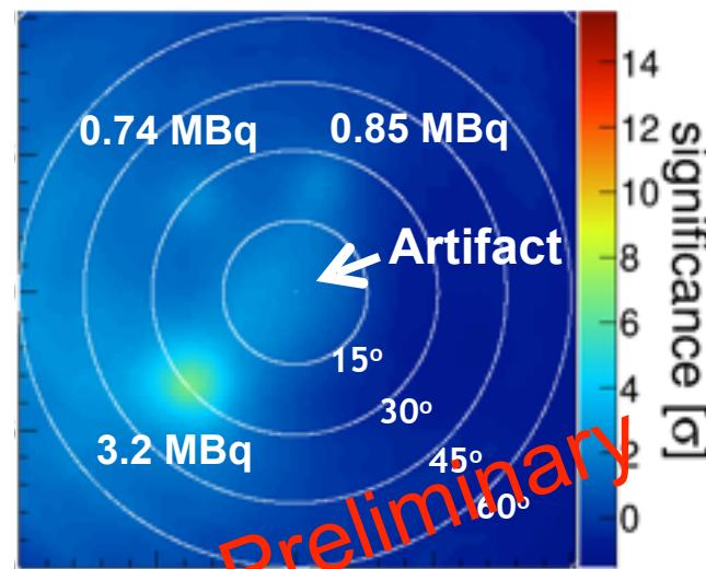
Electron tracks provide 4 times better S/N than usual Compton imaging !
