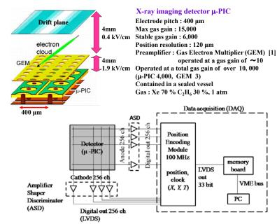
√The output charges of the 256+256 channels are parallel pre-amplified, shaped, and discriminated by the ASD chips.
