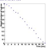
Dehydration reaction of a pyromellitic acid hydrate occurs when heat is applying. A weight fraction of the dehydrate, x, was observed for 20 s using a  $\mu$ -PIC. The intensity  $I(2\theta,t)$  is expressed as  $I=xI_d(2\theta)+(1-x)I_h(2\theta)$ , where  $I_d(2\theta),I_h(2\theta)$  is the intensity of the dehydrate, the hydrate, respectively, including a background.
