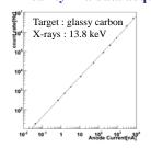
The DAR and the leakage current show a good linear correlation from 20 cps to 5 Mcps (over 10<sup>5</sup>).
